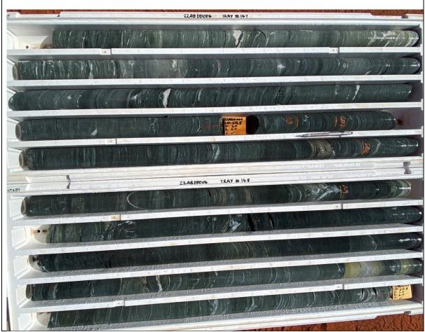
Figure 3 – 22ABDD006 (603.5m – 612.8m) drill core showing sheared mafic with quartz veining and alteration
