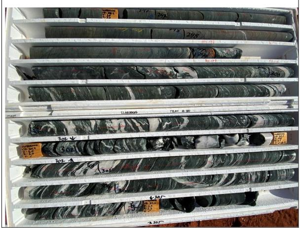
Figure 2 – 22ABDD006 (296.8m – 305.2m) drill core from showing shearing and abundant quartz veining as part of the East Lode intercept.
