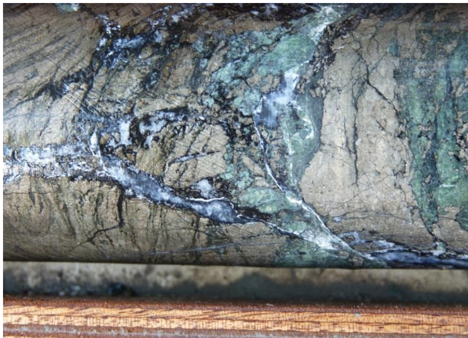
Figure 1: Close-up of high grade copper sulphide mineralisation in LMD001; 30.25-30.35 m.
